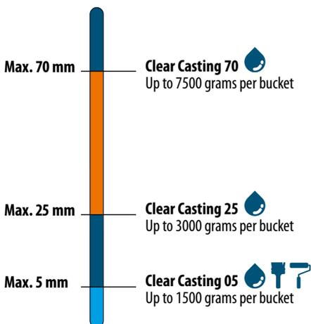
Please note: The maximum pour thickness is an indication to prevent flash cure and applies at 20°C. If the temperature is higher than 20°C, the maximum pour thickness does not apply. For example, when the processing temperature is around 28°C, the maximum layer thickness will be halved. Keep this in mind when working on large projects. If in doubt, contact us.
