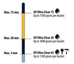
Please note: The maximum pour thickness is an indication to prevent flash cure and applies at 20°C. If the temperature is higher than 20°C, the maximum pour thickness does not apply. For example, if the processing temperature is around 28°C, the maximum layer thickness will be halved. Keep this in mind when working on large projects. If in doubt, contact us.
